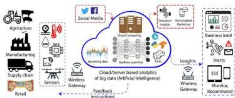
Fig. Pictorial representation of the IoT framework within agri-food industry context.
